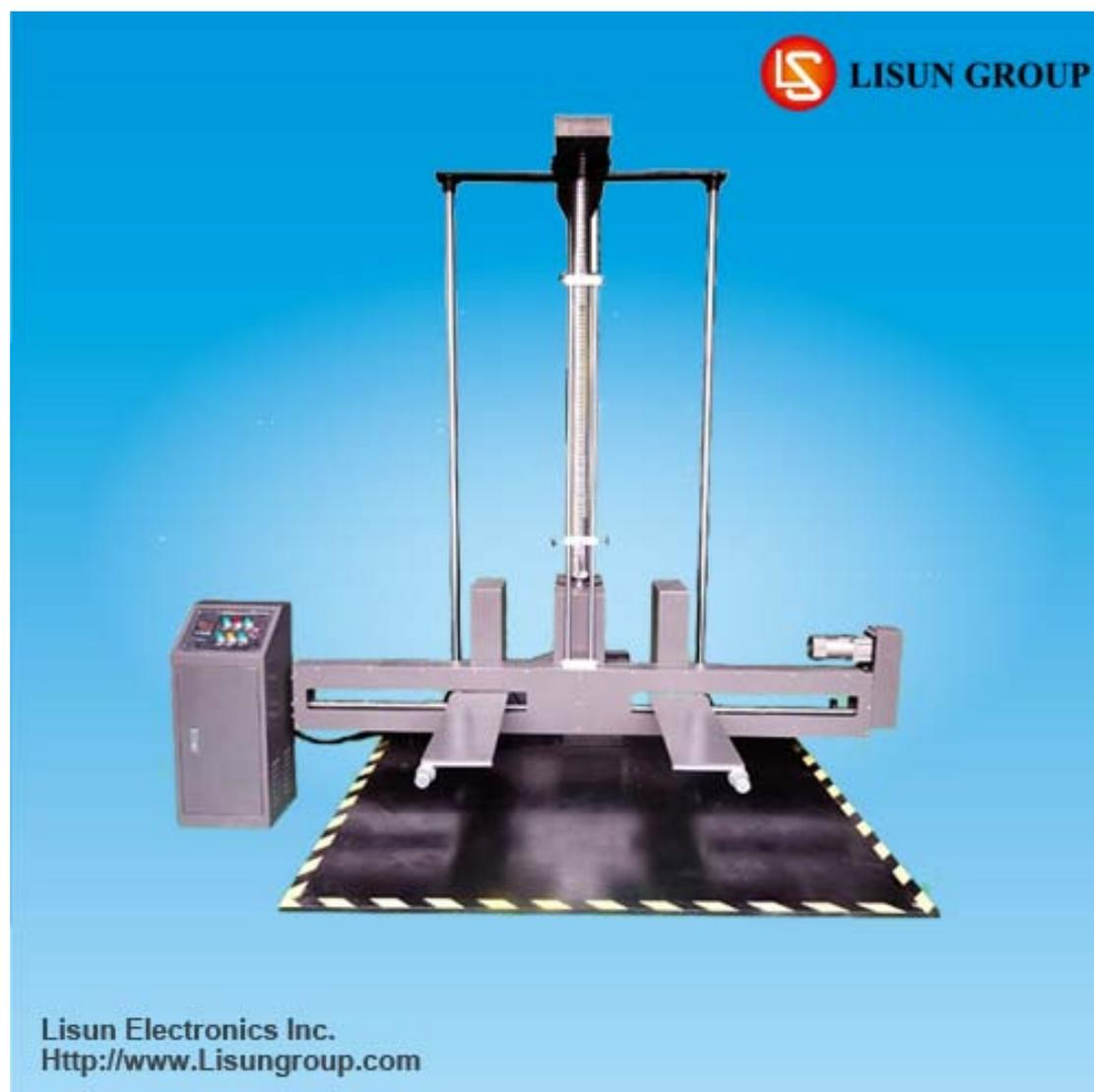
This series drop test bench for measuring the main simulation packages in the transportation, loading and unloading process under drop impact influence, identification package impact strength and packaging design.
