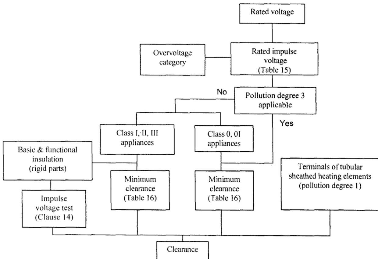
FIG. L-1 SEQUENCE FOR THE DETERMINATION OF CLEARANCES
