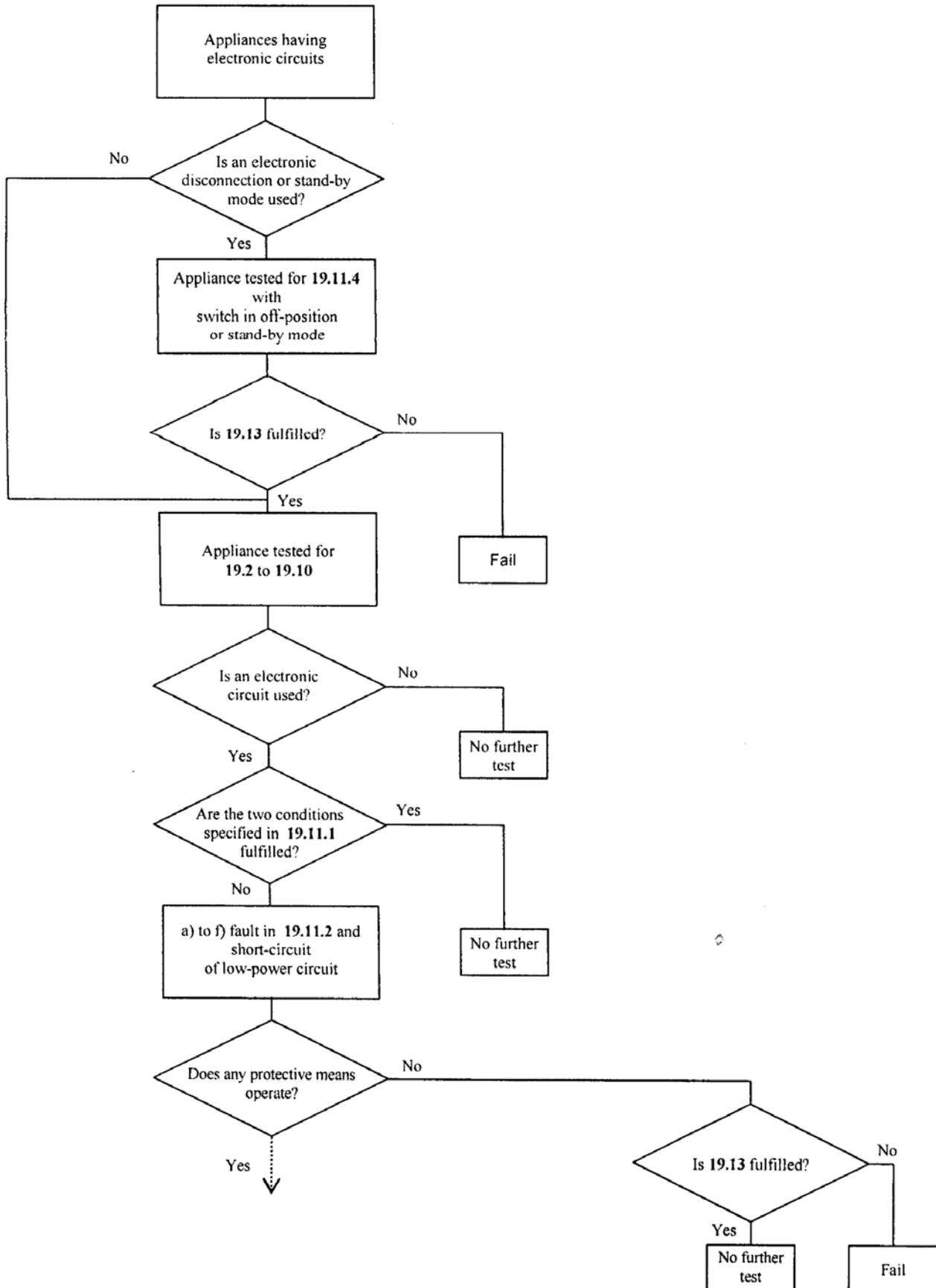
SEQUENCE OF TESTS FOR THE EVALUATION OF ELECTRONIC CIRCUITS — (Concluded)
