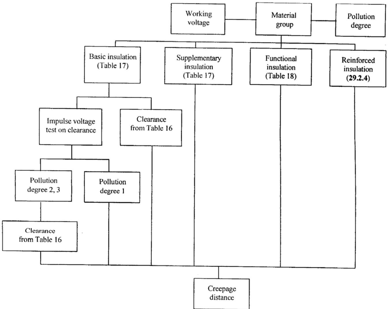
FIG. L-2 SEQUENCE FOR THE DETERMINATION OF CREEPAGE DISTANCES
