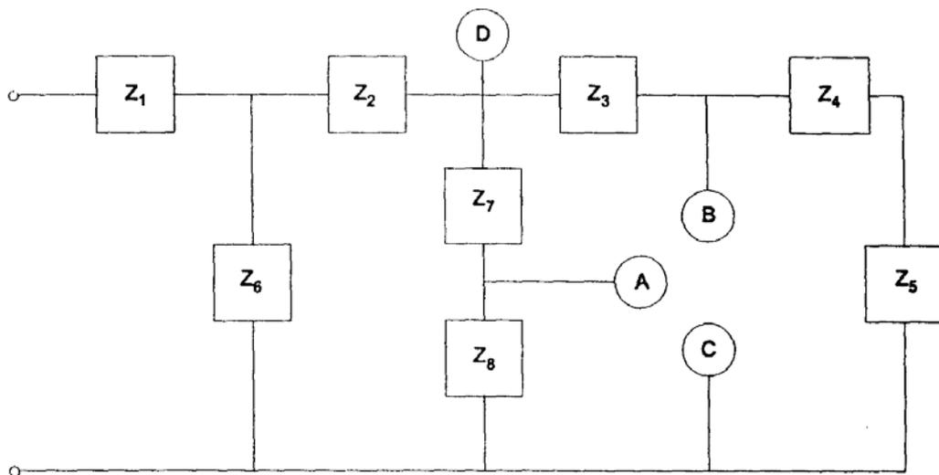
D is a point farthest from the supply source where the maximum power delivered to external load exceeds 15 W. A and B are points closest to the supply source where the maximum power delivered to external load does not exceed 15 W. These are low-power points.
