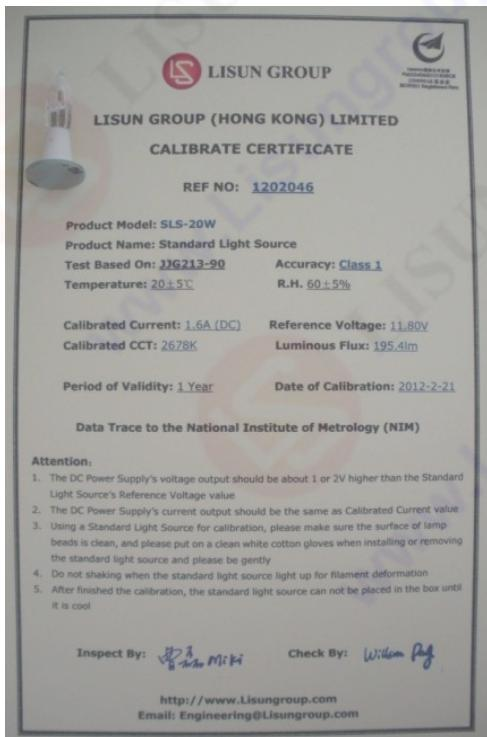
The **Standard Light Source** is used to calibrate LISUN LPCE-2 Scientific Grade Spectroradiometer Integrating Sphere System or LPCE-3 CCD Spectroradiometer Integrating Sphere Compact System. The Standard Light Source Calibrate Certificate can be traced to NIM and NIST. The different size of Integrating Sphere should choose the right power of standard lamp source.
