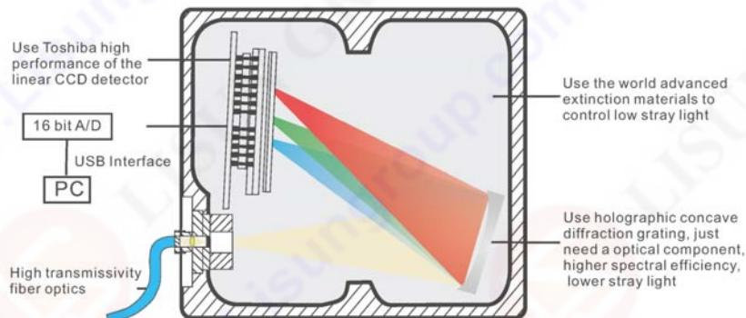
LMS-9000C used the Band pass-filter Wheel Correcting Technique, Spectrometer & Broadband-radiometer & photometer Combined Technique, and modified NIST stray light correction technology, the LMS-9000C Spectroradiometer can realize ultra low stray light and super photometry linearity in overall dynamic range.
